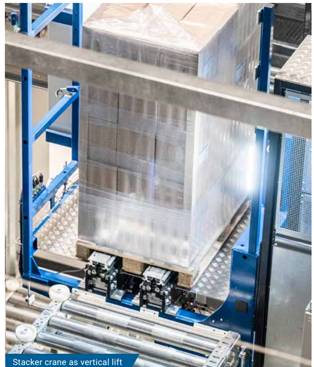
Stacker crane as vertical lift
