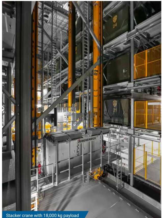
Stacker crane with 18,000 kg payload
