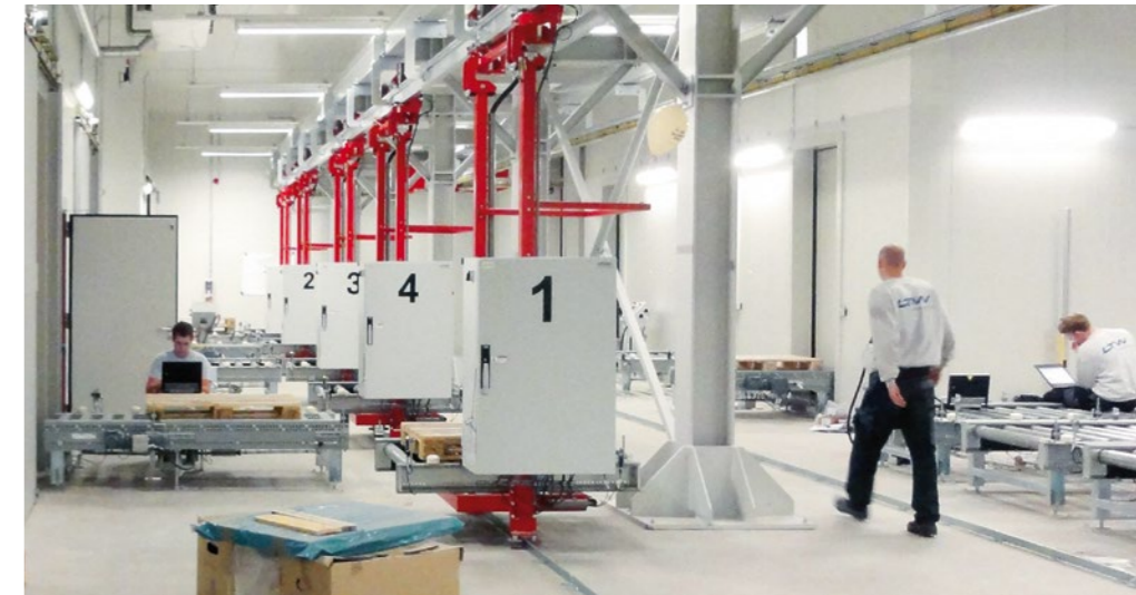
Integration of an electric monorail system (EMS) by the LTW team. The main advantage of the EMS lies in the scalability – in case of a prospective expansion, vehicles can easily be added, during reduced system operation disengaged, for repair purposes separately moved into the climatized maintenance area.
