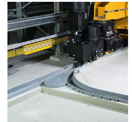
The stacker crane works the switch during driving – without hesitation, monitoring or complex construction.
