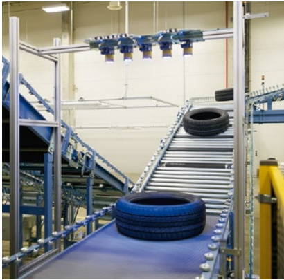
Scanning portal with five cameras working in parallel: Per tire, there are only a few milliseconds available to reliably detect the barcode.
