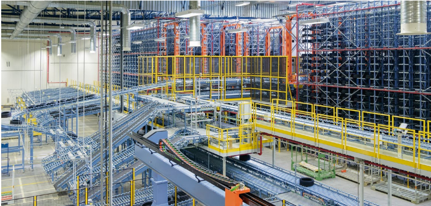
The two wings of the 10 m-high, uncovered high-bay warehouse with central interface to the conveyor system. On the left the discharge conveyors for order picking.
