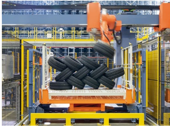
The new palletizer robots used for delivery to resellers calculate the customer-specific pallet stack based on the individual dimensions of each tire model.
