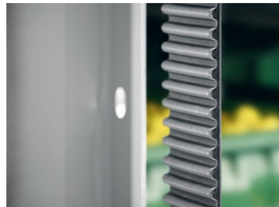
Five years warranty: The origins of the timing belt in the lifting drive of the stacker crane stem from an LTW-cooperation with the research partners ContiTech and SynchroTech.
