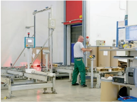
Pre-zone of the high-bay warehouse with I-point (identification point). In the scope of retrofitting, the system communication is converted from Interbus to Profinet.
