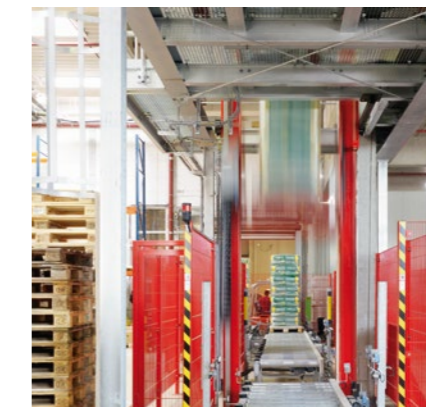
The automatic conveyor line for full pallets consists of three vertical conveyors (see image), two transfer cars and gravity roller conveyors.
