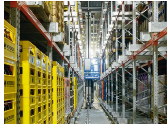
Stacker crane with double-depth telescopic fork on the ground floor. The single-masted design allows reduced run-out and hence provides about 80 additional pallet spaces.
