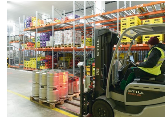
LTW equips the forklift trucks at the outbound area with a camera for automatic label scanning, including WLAN connection to the warehouse management system.
