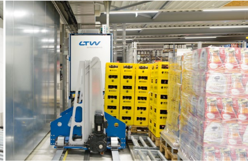
A vertical lift (left) connects the goods entry and exit on the ground floor, the order picking upstairs and the cellar for wines, 3,000-liter beer tanks and other slow-moving items. At the interface to the order picking area, the transfer car (right) docks perfectly to the gravity roller tracks, thanks to the lifting and tilting device. As with the stacker cranes, vertical lift and transfer car are equipped with the patented LTW belt technology.
