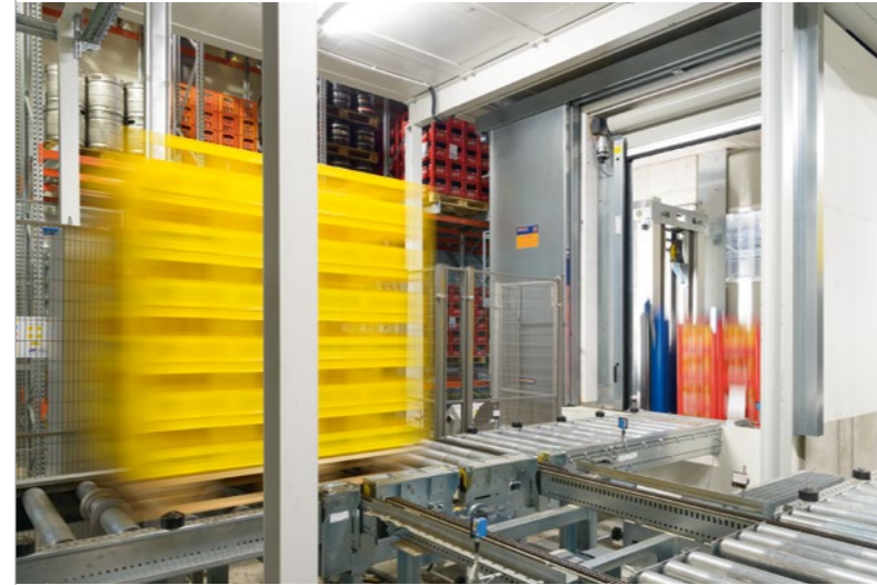
A vertical lift (left) connects the goods entry and exit on the ground floor, the order picking upstairs and the cellar for wines, 3,000-liter beer tanks and other slow-moving items. At the interface to the order picking area, the transfer car (right) docks perfectly to the gravity roller tracks, thanks to the lifting and tilting device. As with the stacker cranes, vertical lift and transfer car are equipped with the patented LTW belt technology.
