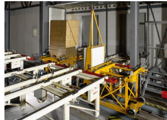
As from 2007, the new and quicker double transfer carriage eliminates a bottleneck in the conveyor technology and, due to a preventive maintenance, runs since then without any problems.
