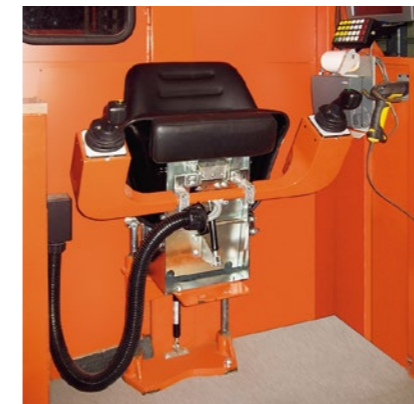
The newly developed folding seat with swivelling joysticks can also be used as a fixed-seat, ergonomic workstation in the order picking area of the warehouse.
