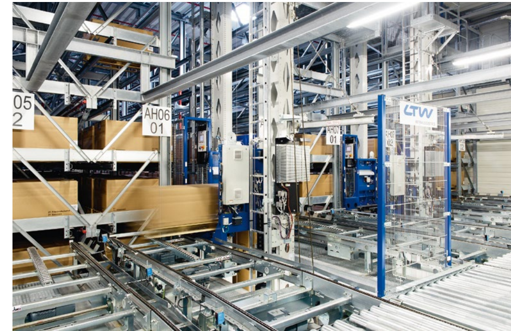
The eight aisle-bound LTW stacker cranes are equipped with service friendly details – such as a lifting assistance for changing heavy components or a video camera on the lifting device for quick and goal-oriented fault analysis.
