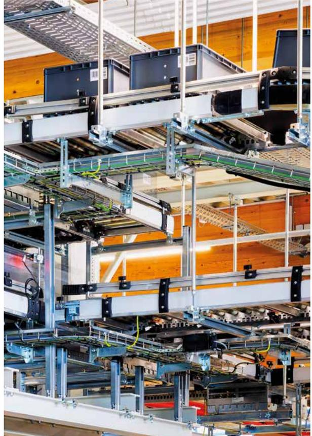
« **A linked up conveyor system is essential when you have a warehouse complex with two separate high-bay warehouses. In our case, the extensive conveyor system with 18 goods-in stations, 16 picking stations, 20 packing stations, and 9 vertical conveyors more than meets our requirements.**
