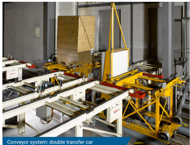
Conveyor system: double transfer car
