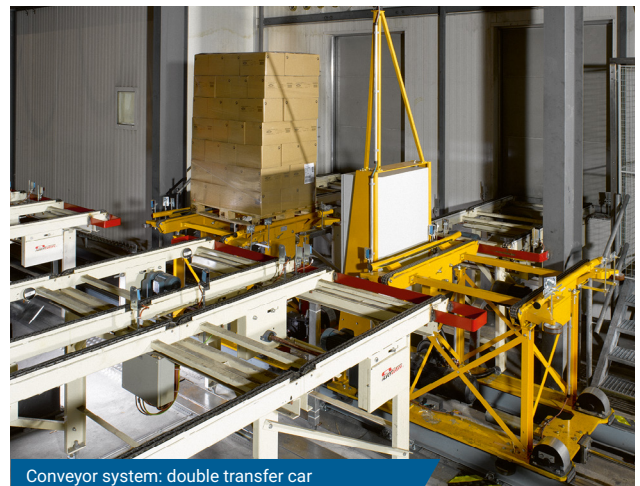
Conveyor system: double transfer car
