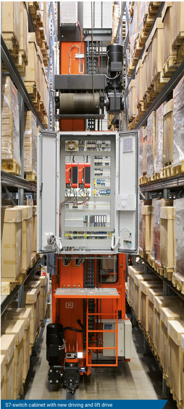
S7-switch cabinet with new driving and lift drive
