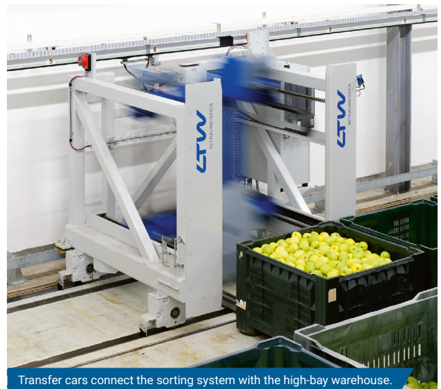
Transfer cars connect the sorting system with the high-bay warehouse.
