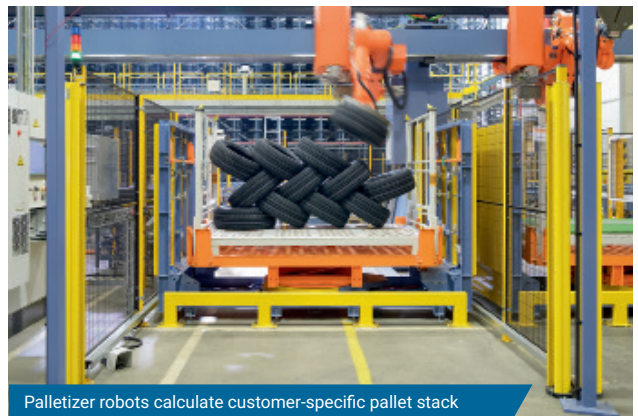
Palletizer robots calculate customer-specific pallet stack
